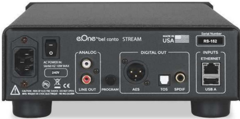
ABOVE: Digital ins are limited to USB-A (for an external memory stick or hard drive) and RJ45 (network). Outputs, selected by the 'Program' button include AES (XLR), optical and coaxial digital plus fixed-level single-ended analogue audio on RCAs
