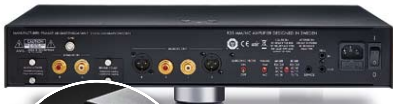
ABOVE: Single phono inputs [far left] are switched between MM/MC by a toggle, alongside other toggles for gain and subsonic filtering. Input loading DIP switches are hidden behind small panels [inset]. RIAA eq'd outputs are offered on RCAs and balanced XLRs
